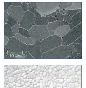
[Figure 2a] > Structure of Al<sub>2</sub>O<sub>3</sub> ceramics.
