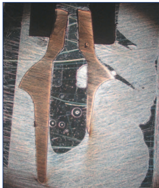
✦ [Figure 7b] Translucence of Ankylos® CERCON® abutment. Thin-ground section 50x magnification.
