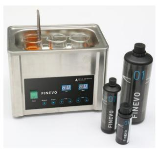
Figure 3. Ultrasonic cleaning protocol. Three times ultrasonic bath at 30°C for 5 min each. 1) antibacterial FINEVO cleaning solution; 2) 80% ethylalcohol; 3) aqua dest.
