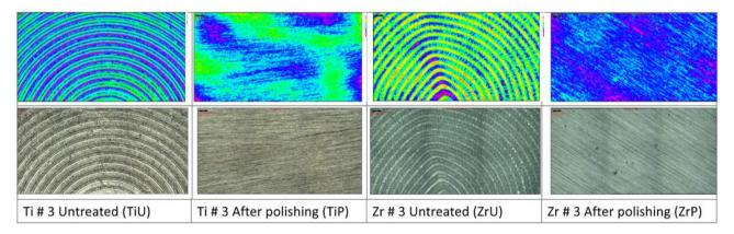
Figure 4. Profilometric example images of height display color scale (top row) and true color representation (bottom row) of untreated and Panther polished titanium and zirconia test specimens.
