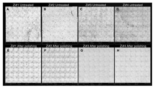
Figure 6. SEM pictures ( $500\times$ ) of untreated zirconia disk specimens (A-D) with visible contamination particles and circular milling grooves from CAD/CAM machining. Reduced surface contamination with scattered residues and surface leveling after 2-step polishing procedure with Panther polisher (E-H) ( $500\times$ ).
