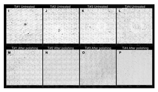
Figure 5. SEM pictures ( $500\times$ ) of untreated titanium disk specimens (I-L) with contamination particles of different size and centric milling grooves from CAD/CAM machining. Debris to a different extent and surface smoothing effect after a 2-step polishing procedure with Panther polisher (M-P) ( $500\times$ ).
