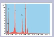
**Figure D5** XRM-analysis showing presence of calcium and phosphorus.
