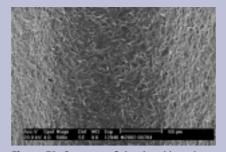
**Figure F2** *Structure of titanium-blasted surface.*
