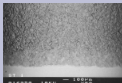
Figure B1 Surface of grit-blasted and acid etched implant.
