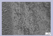
**Figure C2** Topography of surface produced by anodic oxidation; porous structures.
