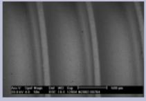
**Figure D1** Inhomogeneous porosities on threads.
