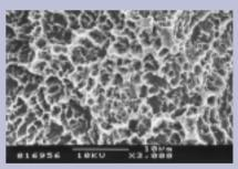
**Figure B3** Homogeneous topography of gritblasted and acid-etched surface.
