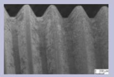
**Figure C1** Inhomogeneous surface morphology, produced by anodic oxidation.
