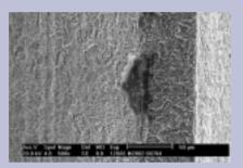
**Figure A4** *Embedded particle; magnification* 500x.
