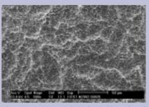
**Figure B2** Topography of grit-blasted and acid-etched surface.
