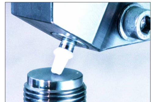
Fig. 2: Close-up of dynamic strength testing of implant-zirconium-dioxide-abutment assembly.
