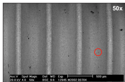
Embedded particles on surface
