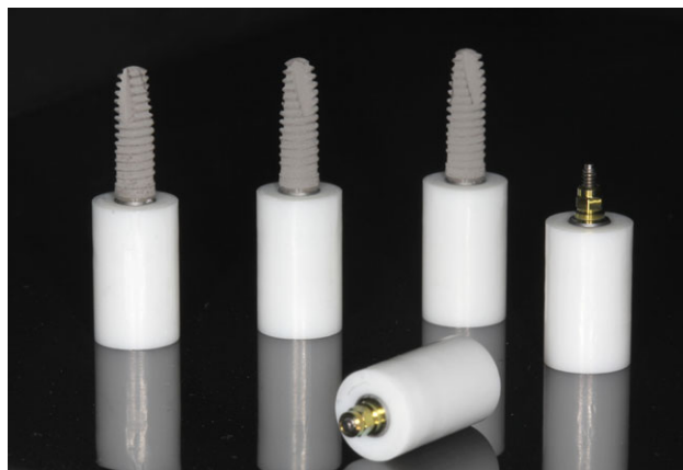
Figure 1 Test specimens: two-piece zirconia abutments connected to internally hexed implants. Zirconia copings were modified for the test setup.
