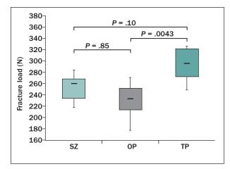
**Fig 8** Fracture loads of abutments in the three groups. Shown are 10th percentile (lower whisker), 25th percentile (lower box margin), median (center line), 75th percentile (upper box margin), and 90th percentile (upper whisker).
