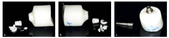
Figs 7a to 7c Types of failure of the abutments. (a) Prefabricated (SZ #4), (b) OP CAD/CAM (#3), (c) TP CAD/CAM (#3). Note the bent screw at the TP abutment.
