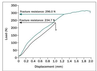
**Fig 5** Examples of load-displacement diagrams of SZ (#7) and TP (#4) abutments. In the SZ (one-piece) abutment, the maximum recorded force equals the fracture resistance (here, 234.7 N), whereas in the TP abutment, the fracture resistance reading can be taken at the transition from the quasilinear to the flattened, more irregular curve.
