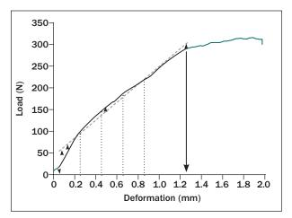
**Fig 6** Schematic stress-strain diagram (TP #3). Black field = reversible elastic deformation; green field = irreversible plastic deformation. The black arrow at right indicates the transition from elastic to plastic deformation.
