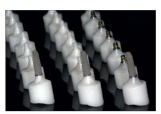
**Fig 3** Twenty-one geometrically identical, simplified zirconia crowns (CERCON) for the allocated control and test abutments (Xive S, 3.8 mm in diameter).
